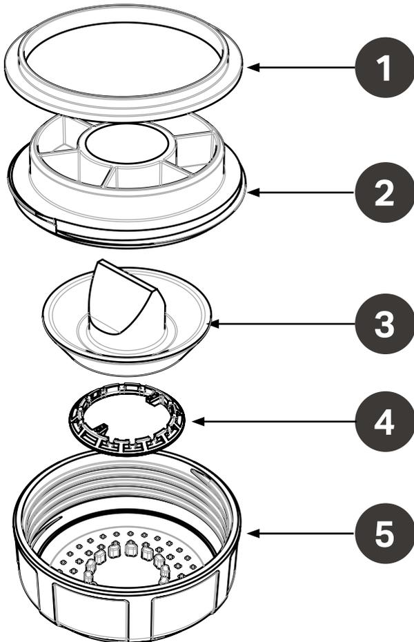
The VAAST Auto Breather Cap is a two-way valve that lets air in while draining the tank and air out while filling the tank.
