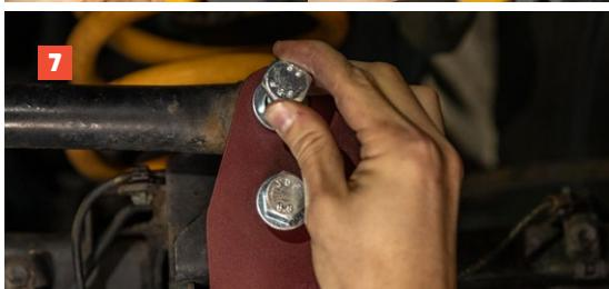
**Non-KDSS vehicles:** the outer bracket needs to sit between the Panhard mount and sway bar.
